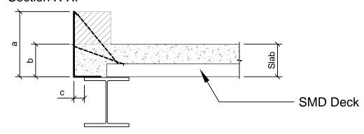
Where edge trim height is requested between 250mm and 450mm high, SMD require 2 sets of restraint straps to minimise the deflection in the face of the trim. One set of straps are required to the top of edge trim (a) at 750mm c/c's and a second set to the middle of the trim upstand (b) at 750mm c/c's staggered between the straps to the top of the trim (As shown above).
