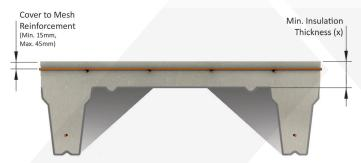
The image and table above details the minimum insulation thickness required to suit fire design criteria in accordance with BS EN 1994-1-2
