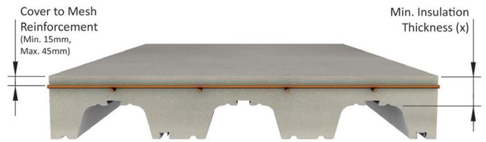
The image and table above details the minimum insulation thickness required to suit fire design criteria in accordance with SCI PN005c-GB or BS5950 Part 8.
